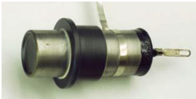
Figure 2. Geiger-Muller Tube. Source: Hudoba 2010
